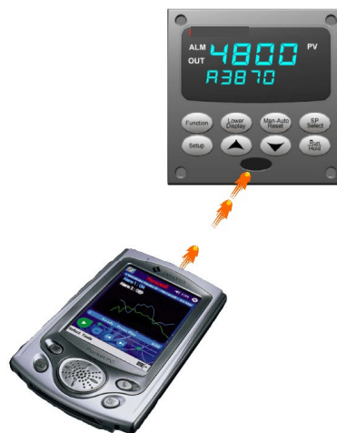
Figure 1-3 Depiction of infrared communications
